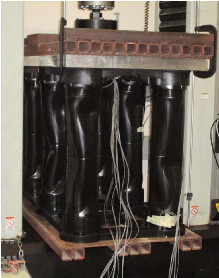
Figure 3: Typical Silva Cell 2X Failure
