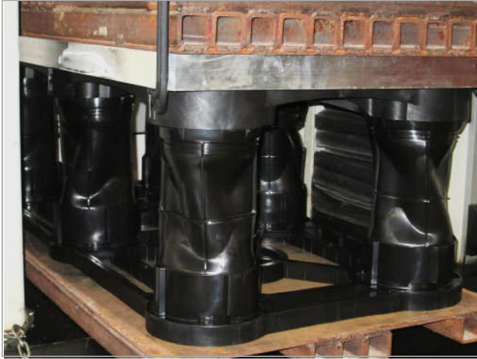
Figure 1: Typical Silva Cell 1X Failure
