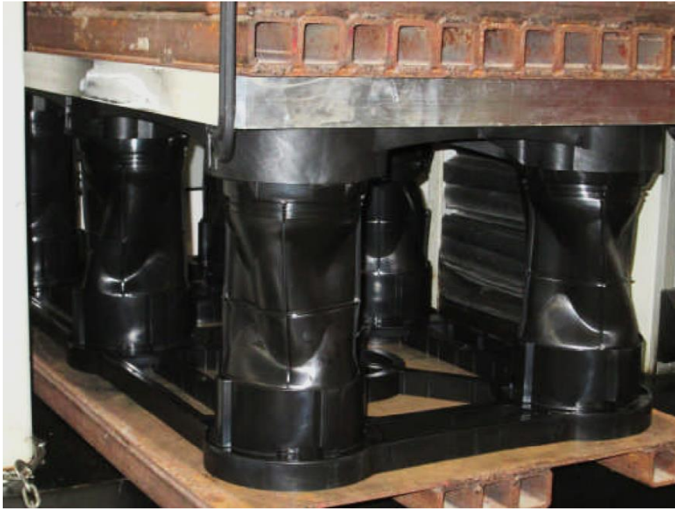
Figure 1: Typical Silva Cell 1X Failure
